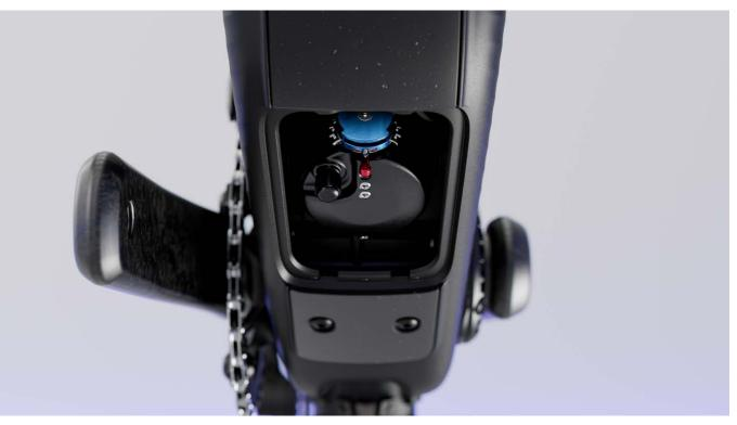
Shock accessibility and user-friendliness was paramount when designing the Voltage. The downtube door that is featured on all Voltage models is super simple to remove, taking just a quarter turn of the dial to remove the cover. The large opening makes things like shock adjustments and cable routing much easier. Additionally, removing the shock is a piece of cake. A window on the drive-side of the seat tube gives direct access to the shock bolt.
